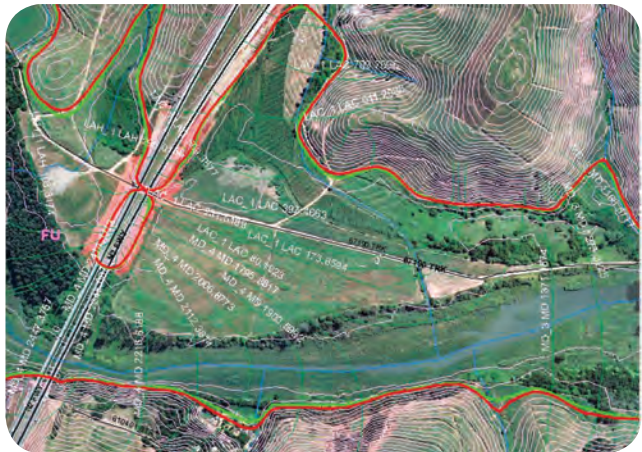
▲ The red-line indicates the setback line for predicted future flooding
