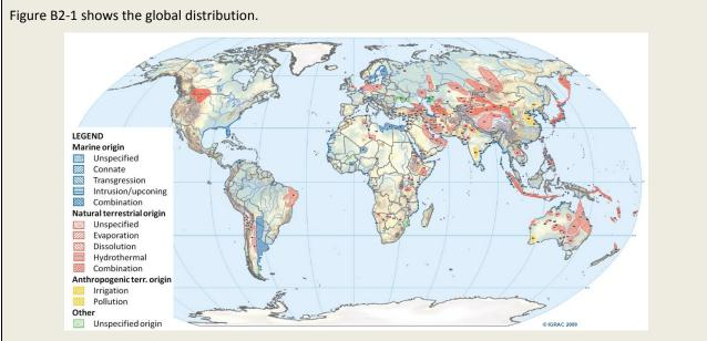
Figure B2-1. World distribution of major reported problems of arsenic content in groundwater at concentrations higher than 50  $\mu$ g/L (Smedley, 2008; Margat and van der Gun, 2012).
