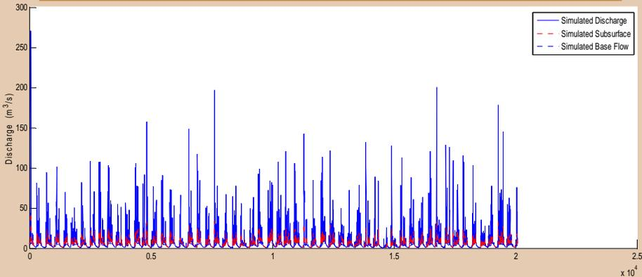
**DREAM simulates the surface runoff, the subsurface runoff and the ground water contribution to streamflow**
