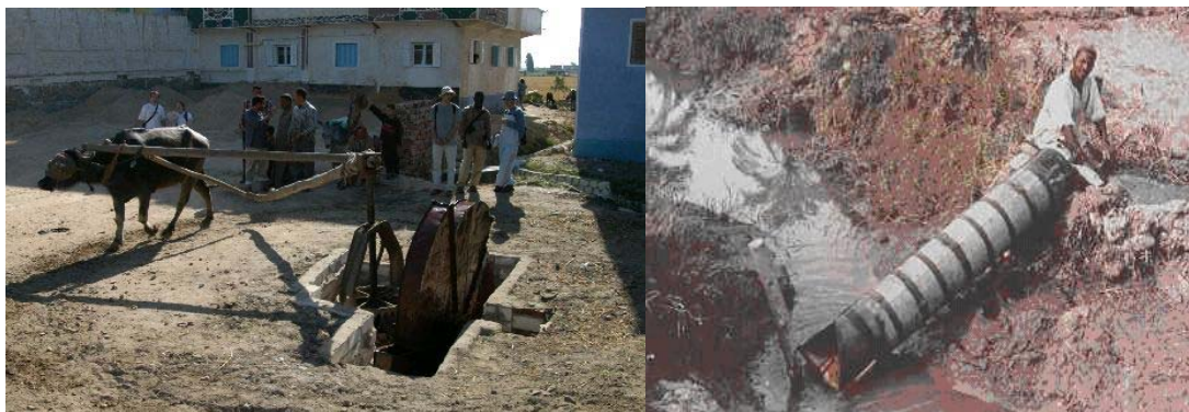
Figure 21. Animal powered Sakya still operating in AlRezqa area until the millennium in areas uncovered by the IIP and the Tanbour used in the past
