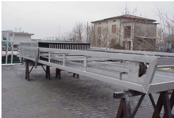
Self Cleaning grid – phase of assembly. Friulana Costruzioni –Italy - December 2007
