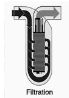
Fig.3: Water filtration movement
