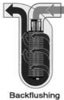
Fig. 8: Water movement during the back-flush operation
