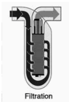
Fig.5: Water filtration movement
