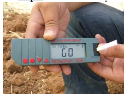
Step 8: Calibrate the strip
