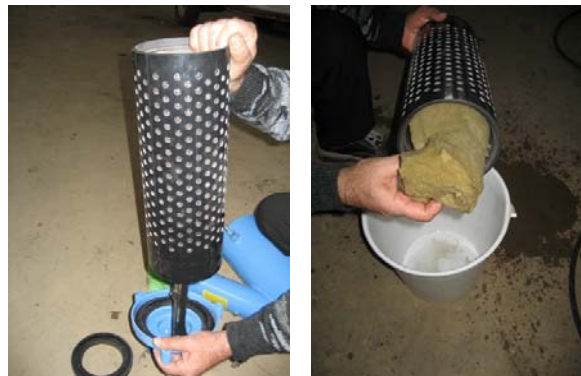
Fig. 5: Manual cleaning of the screen filter. The screen cartridge is firstly withdrawn from the filter body, to operate the necessary scrubbing.
