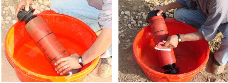
Fig. e: Cleaning of disc filter.
