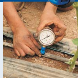
3. Interlogg the needle and the gauge on the basis that is fixed on the pipe
